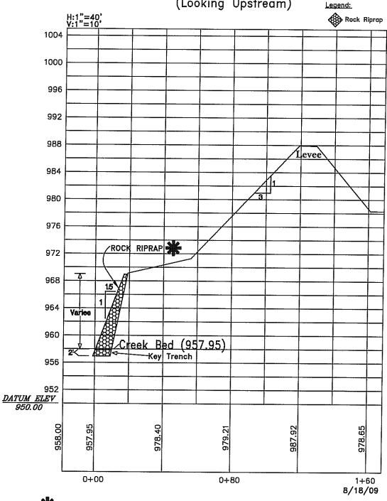
THE RIPRAP SHALL BE COVERED, FROM THE TOP OF THE STRUCTURE DOWN TO THE ANNUAL ORDINARY HIGH WATER LINE, WITH A MINIMUM OF 6 INCHES OF SOIL COMPACTED INTO THE VOIDS OF THE RIPRAP, & IMMEDIATELY SEEDED WITH AN ANNUAL COVER CROP / NATIVE GRASS SPECIES.
